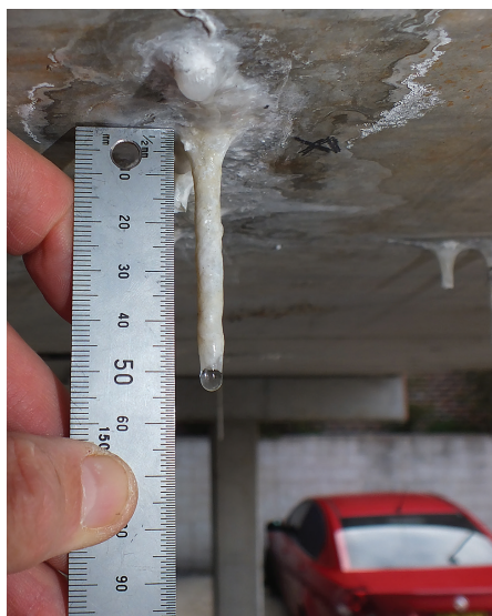
Measuring calthemite straws with engineering metal ruler graduated in 0.5 mm increments
